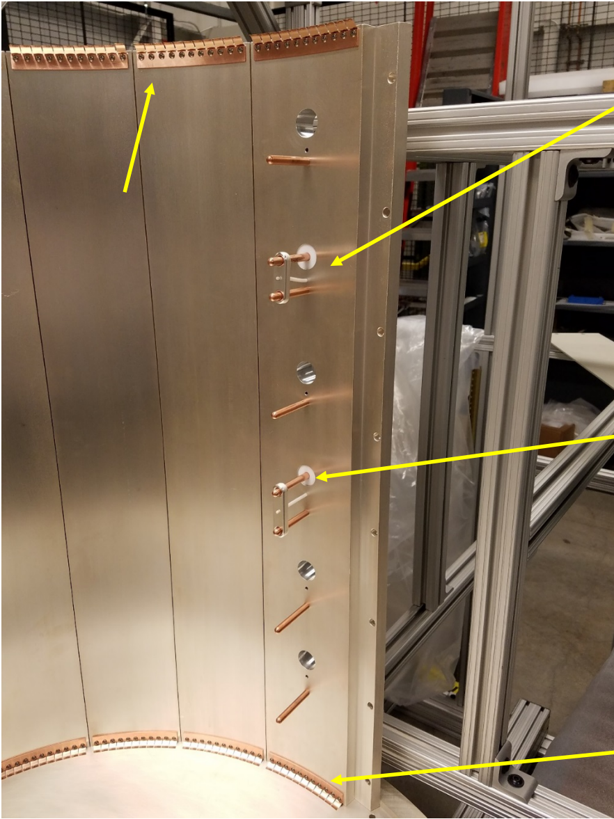
CAVITY INTERIOR SHOWING PANEL FINGERSTOCK AND ADJUSTABLE COUPLING LOOP
