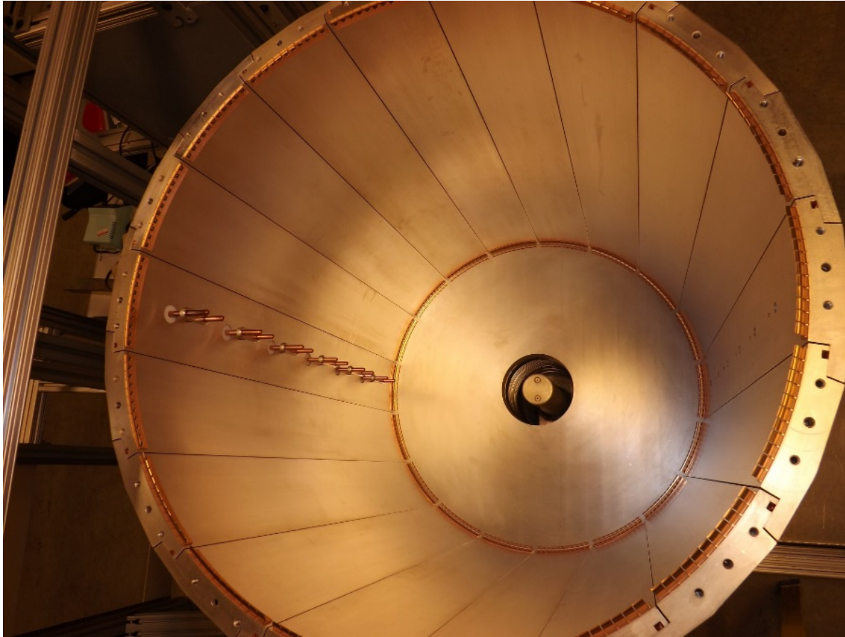
INTERIOR VIEW OF COMBINING CAVITY DURING ASSEMBLY SHOWING SIX INPUT LOOPS ON ONE PANEL AND OUTPUT COUPLING PROBE AT BOTTOM CENTER
