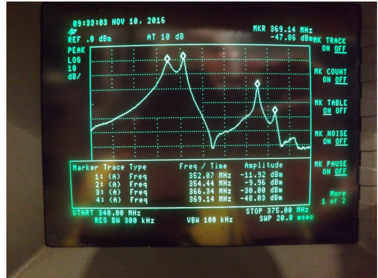
THE CAVITY TUNING PROFILE IS MEASURED USING A LOW-POWER RF SWEEP PERFORMED WITH 77KV/10A BEAM
