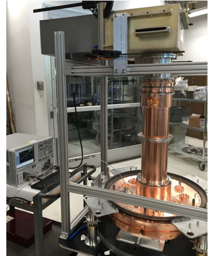
Cold test of MB-IOT output cavity
