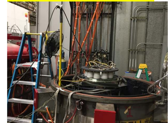
Set up for hipotting grid to anode up to 65 kV
