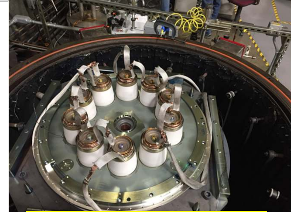
Setup for 25A heater process
