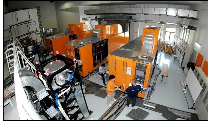
Three 300kW transmitters in Ring for three SRF cavities
