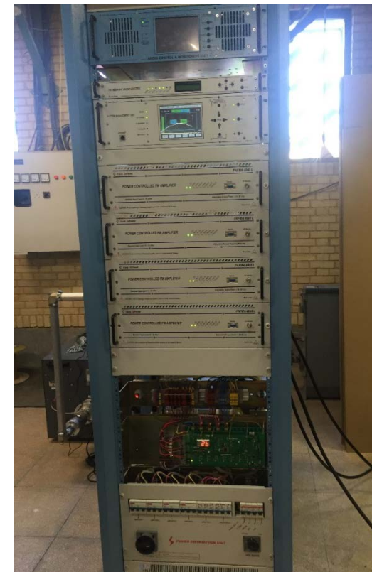
12kW SSA FM transmitter (87.5-108 MHz) 4*3.5kW modules, hot-plug, water-cooled "20kW is in production"
