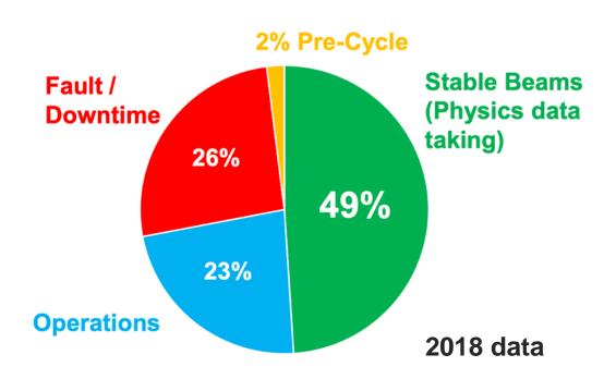
Efficiency very high in spite of the complexity of the machine and the very high stored beam energy (> 300MJ per beam)
