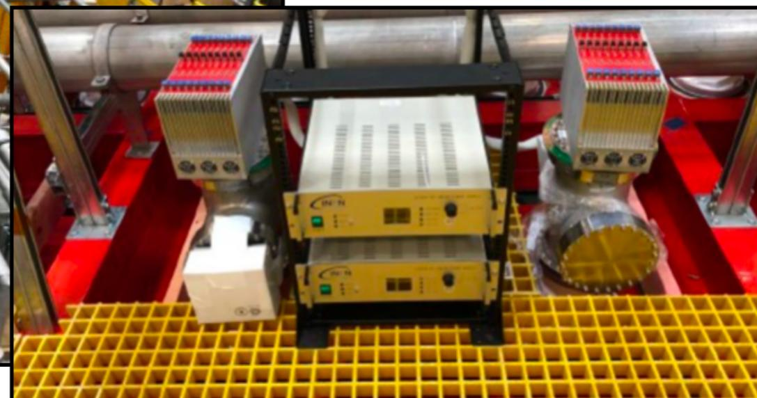
ICARUS commissioned Installed PMT electronics
