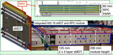
Installation of new triplet RPC chambers in the BIS layer requires replacement of the existing MDT chambers by sMDT chambers to provide sufficient radial space Independent interleaved supports on common rail system
