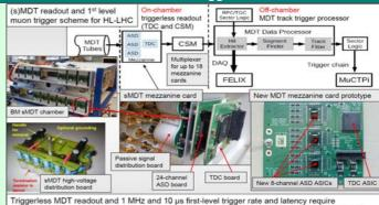
Triggerless MDT readout and 1 MHz and 10 µs first-level trigger rate and latency require — replacement of 20000 MDT and prod. of 2000 new MDT mezzanine cards (prototypes exist), 64 FPGA-based first-level muon track trigger processors, performing pattern recognition and track & momentum reconstr. within 300 ns at HL-LHC bg. rates (demonstrated on prototype HW)
