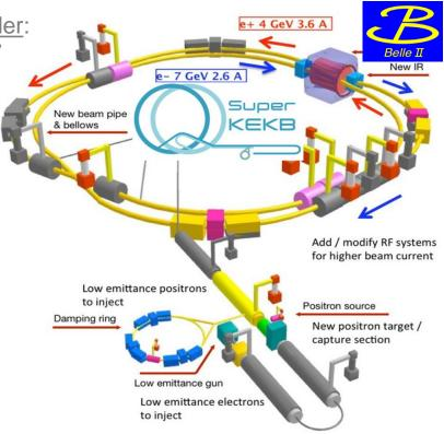
SuperKEKB: second generation B-Factory. It will provide the *world highest luminosity*, applying the *large crossing angle nano-beams scheme*. (P.Raimondi et al., arXiv:0709.0451)
