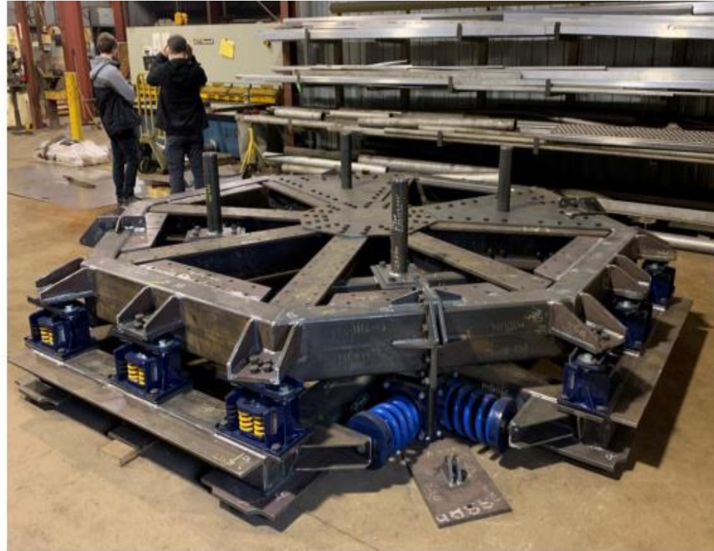
Seismic platform fabricated, shipping to SNOLAB in September
