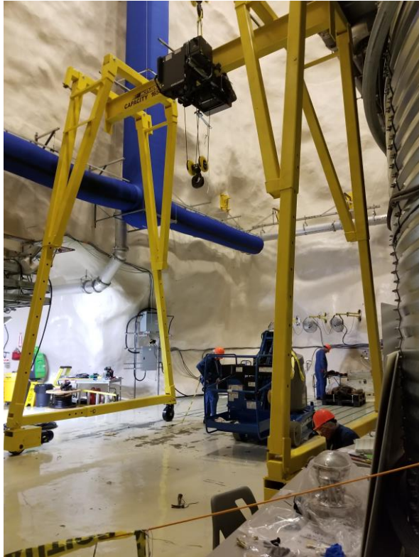
17-ton gantry crane constructed. Commissioning in July
