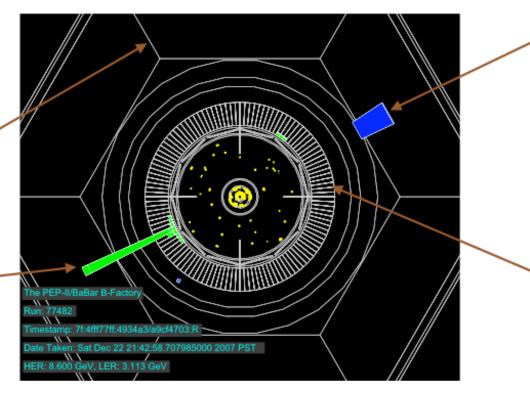
photon shower detected in muon system. Inefficiency produces single photon events.
