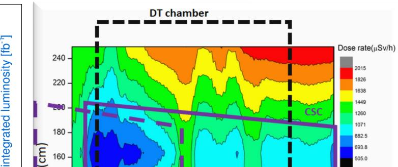
Dose rate just in front of the chamber installed at GIF++. Other detectors under irradiation are placed between the source and the DT chamber. This produces an inhomogeneous irradiation profile on the detector. The dose rate was averaged over the whole chamber to calculate the accumulated dose.
