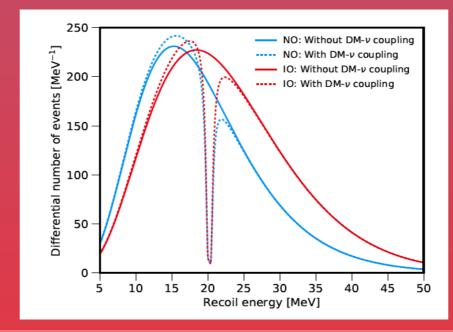
Differential number of electron antineutrinos observed in JUNO for a typical supernova at a distance of 10 kpc, as a function of the detected positron recoil energy[4].
