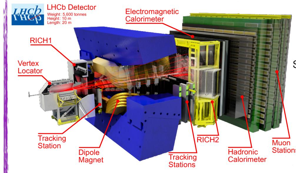
LHCb is a forward spectrometer (2 <  $\eta$  < 5) designed for **B** physics with *proton-proton* collisions
