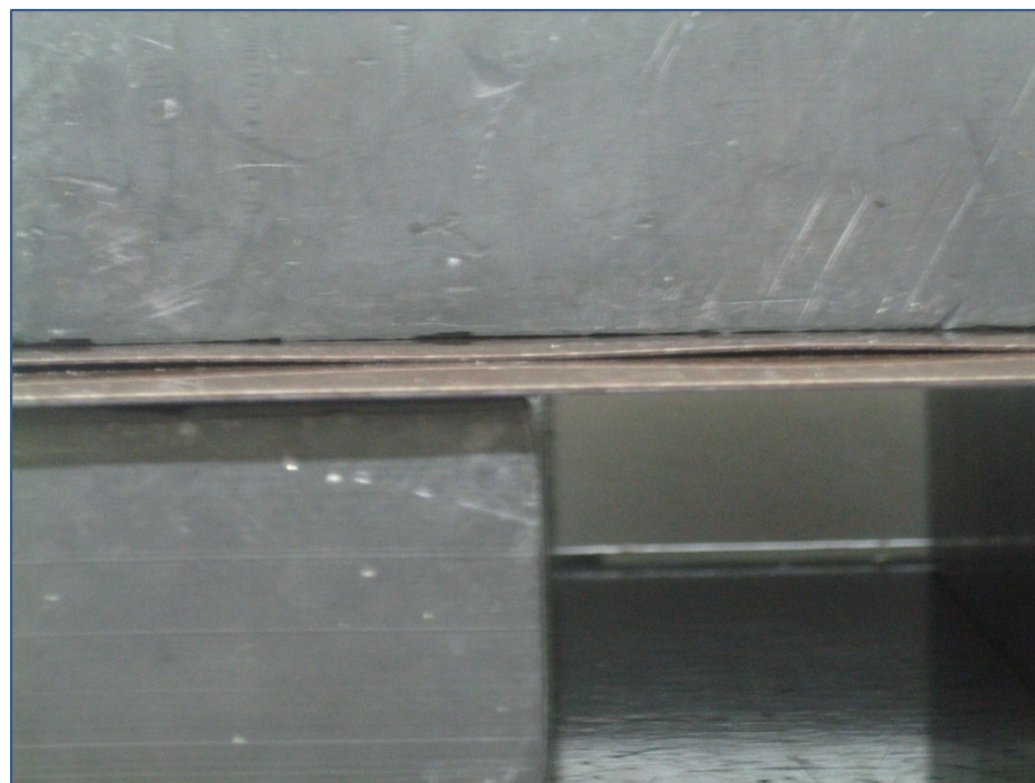
Attached HPLs are not parallel to Each other.
