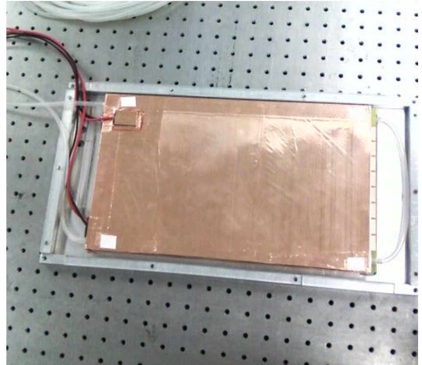
Assembled RPC chamber with 1.0mm HPL.
