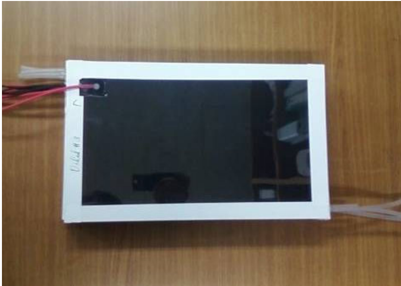
Assembled RPC chamber with 1.0mm HPL.
