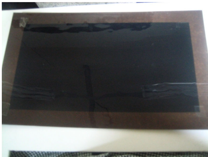
350mm x 210mm HPL with graphite & PET coating
