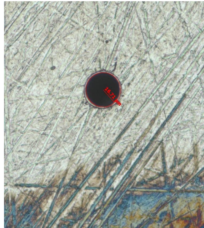
30um hole, mechanically drilled
