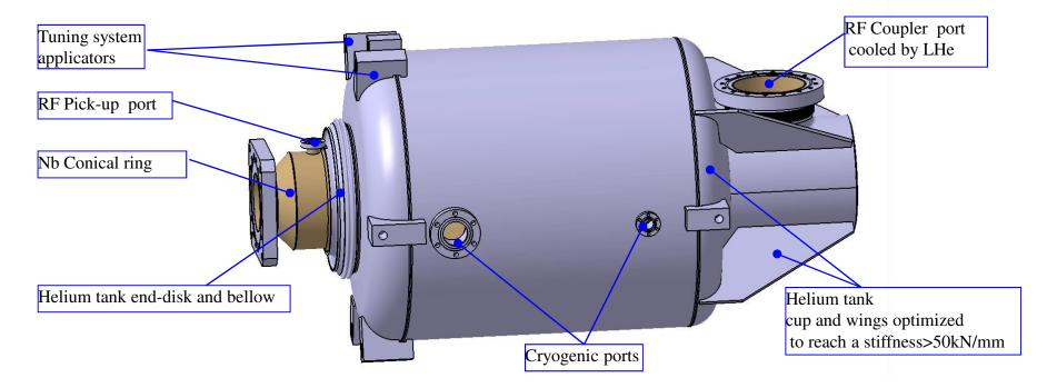
At the end of Phase 2, the cavity is ready for preparation, measurements and cold tests in horizontal cryostat
