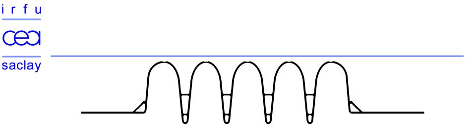
Regulations  $\Rightarrow$  the cavity must sustain twice the maximum pressure
