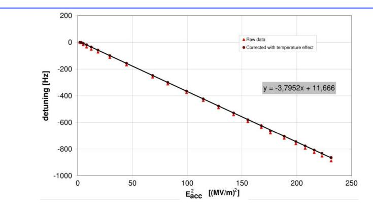
temperature changes during experiment -> pressure changes-> need for a correction of the frequency measurements (black dots)
