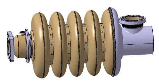
Fabrication of the Niobium cavity
