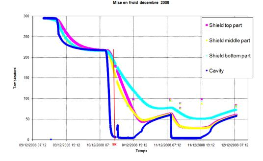
• Bad thermalization: magnetic shield temperature still > 150K when Tcavity is < 9K
