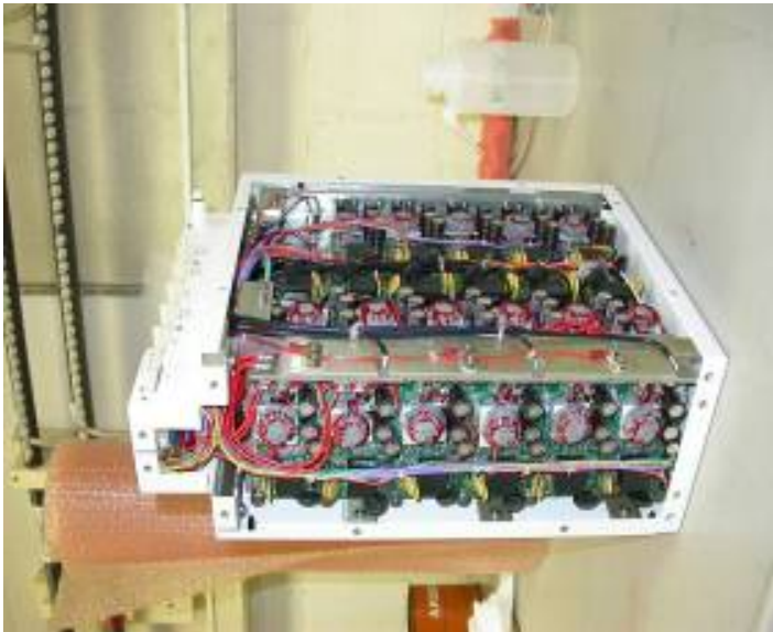
LAr low-voltage power supply
