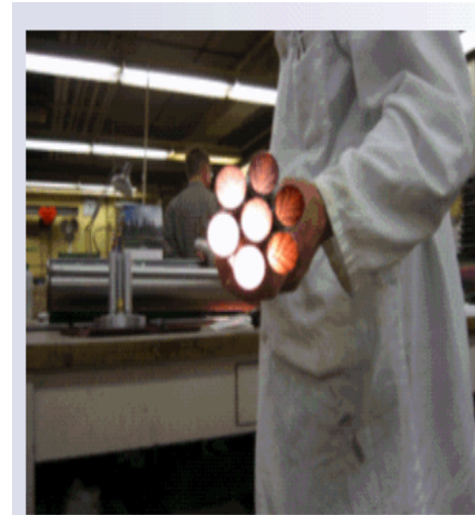
Aluminium Tubes transmitting light (in the final detector these tubes will have 0.5 mm wall thickness)
