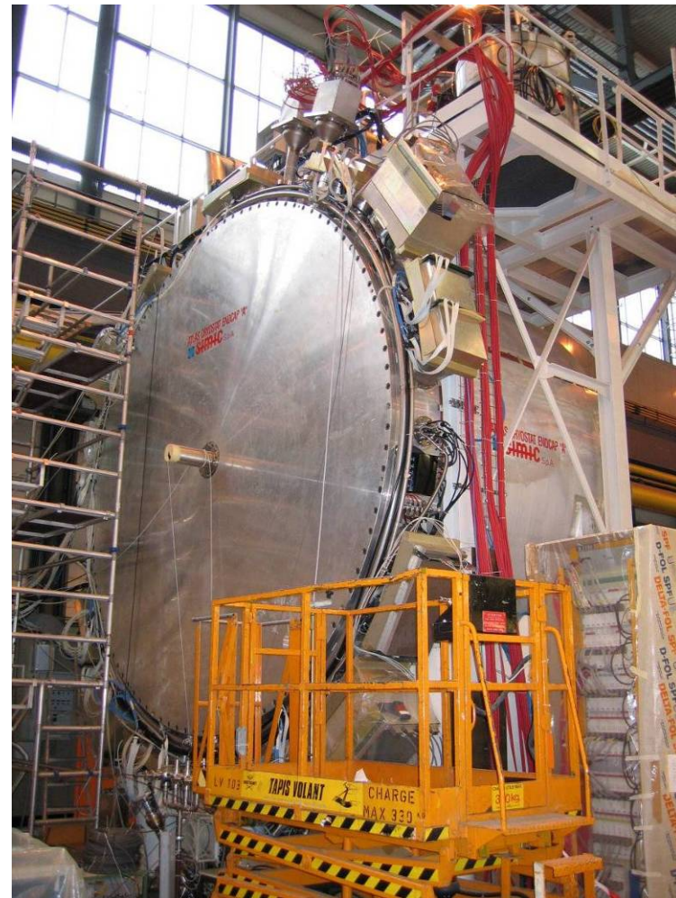
End-Cap A during the surface cold tests
