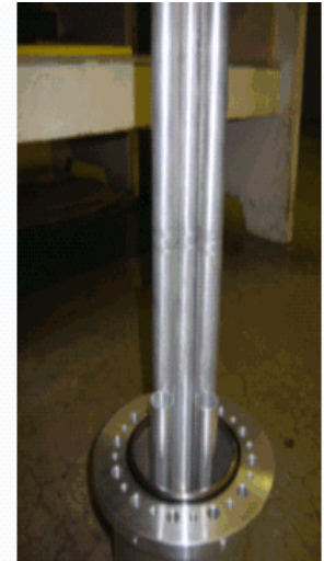
Cherenkov tubes inserted into the Winston cones
