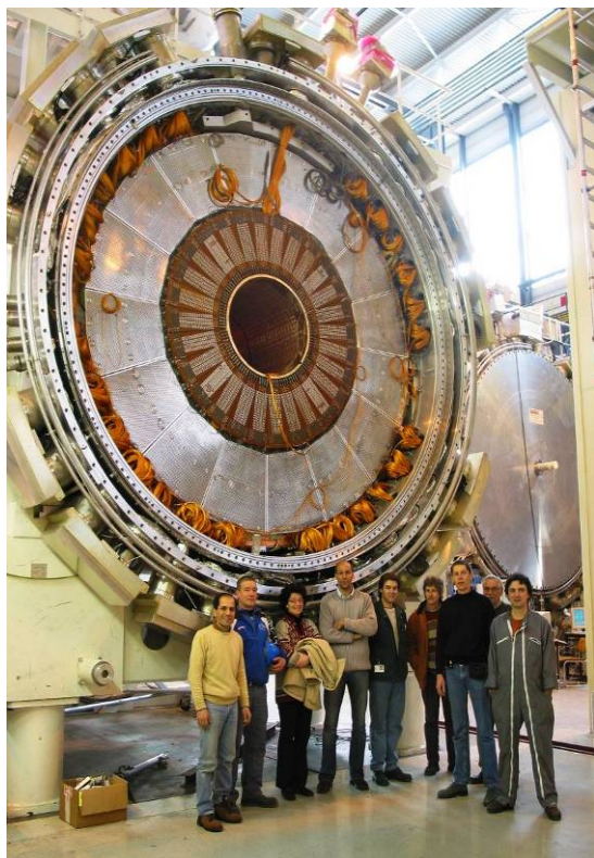
End-Cap cryostat A before the insertion of the FCAL and closure
