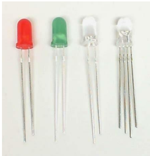
Figure 2-1; Typical LEDs including standard red and green, high-efficiency in various colours, and RGB.
