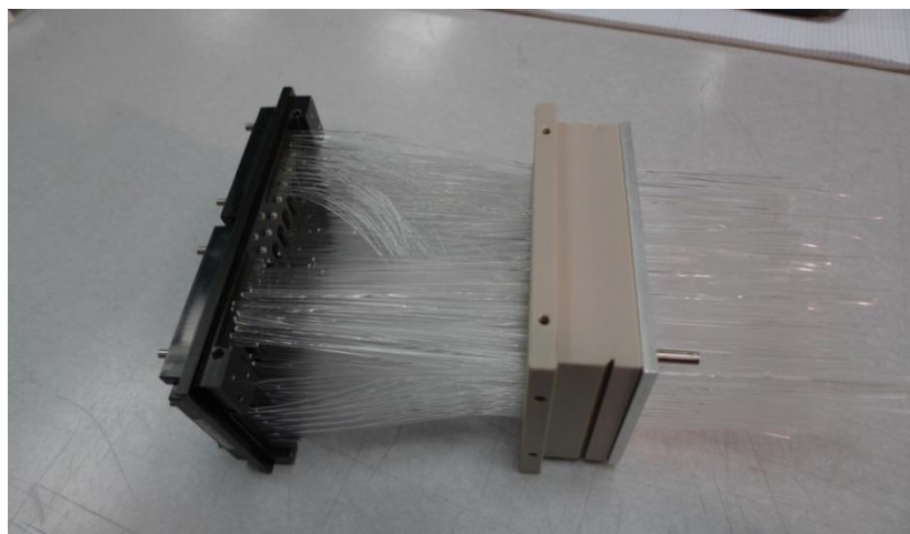
Optical test, glue, flycut the ends
