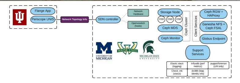
Core Ceph cluster sites share **identical** config and similar numbers / types of OSD Any site can be used for S3/RGW access (HAproxy uses RGW backends at each site) Any site can be used via Globus endpoint (same shared FS) Users at each site can mount NFS export from Ganesha + Ceph FSAL. NFSv4 idmap umich\_ldap scheme used to map POSIX identities.
