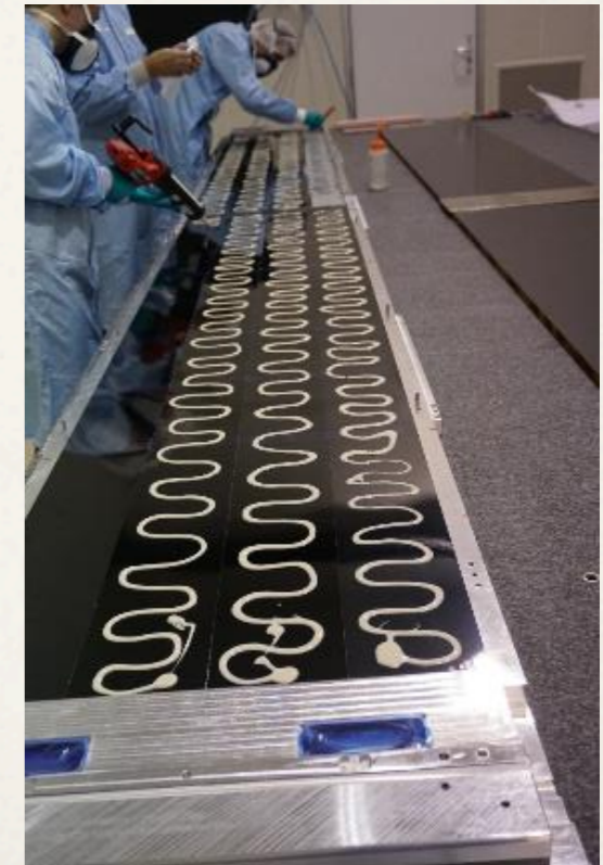
Mats and end pieces positioning, applying glue
