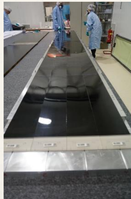
Mats and end pieces positioning, applying glue
