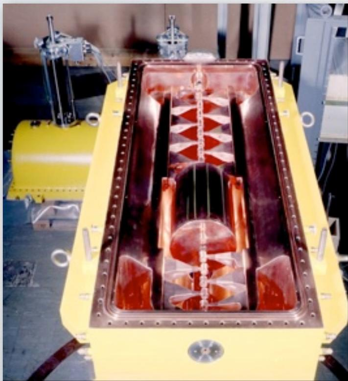
REX IH cavity at CERN/ISOLDE
