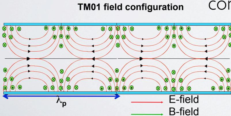
$$k_z^2 = \frac{\omega^2}{v_{ph}^2} = \frac{\omega^2}{c^2} - \frac{\omega_c^2}{c^2}$$
