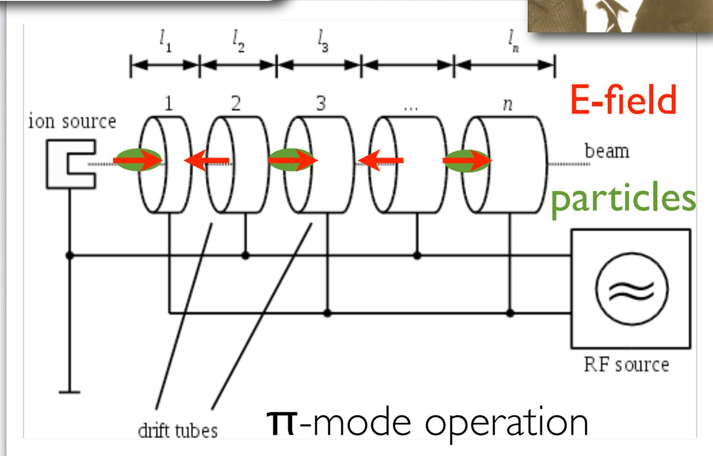
the RF phase changes by  $180^\circ$ , while the particles travel from one tube to the next
