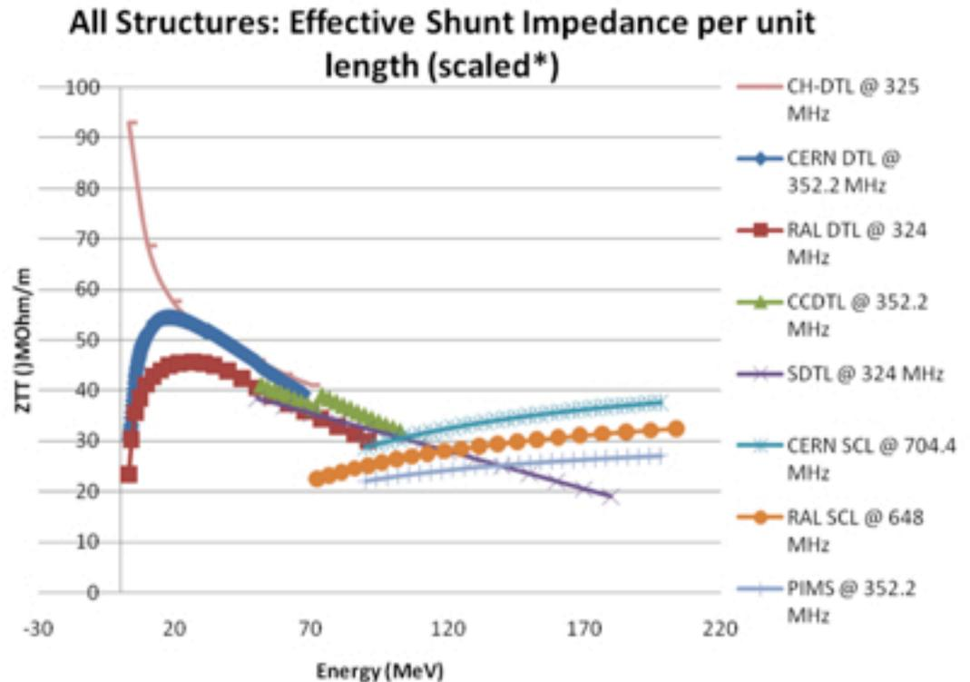
Figure 17. Effective Shunt Impedance per unit length for all structures.
