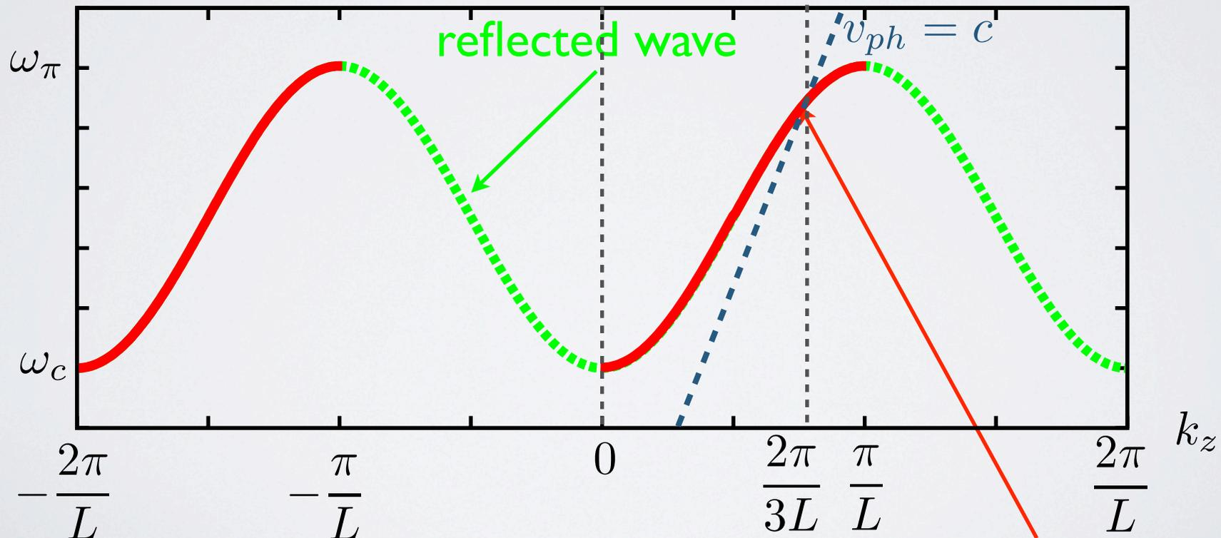
structure with:  $v_{ph} = c$  at  $k_z = \frac{2\pi}{3}$  (SLAC/LEP injector)
