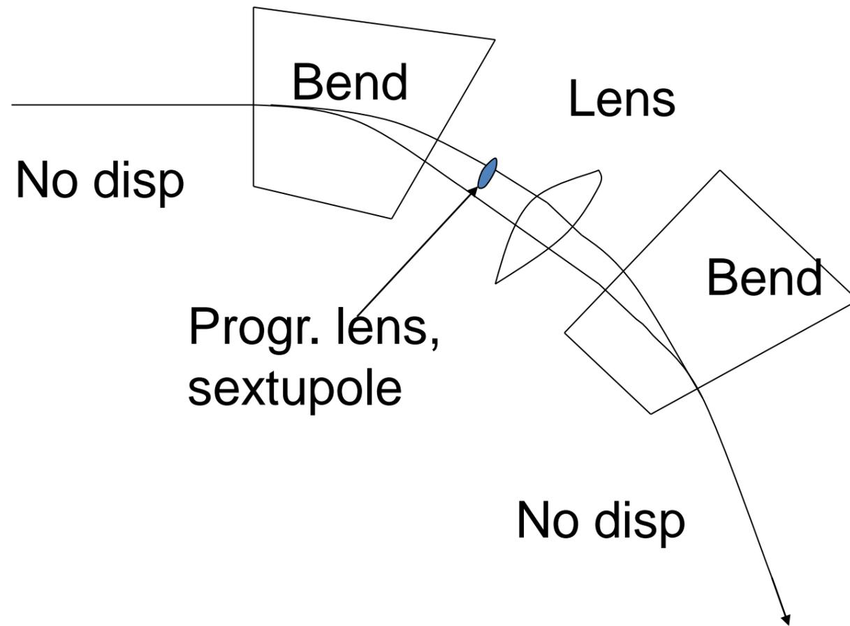
One unit cell consisting of two bending magnets and a focusing lens between.
