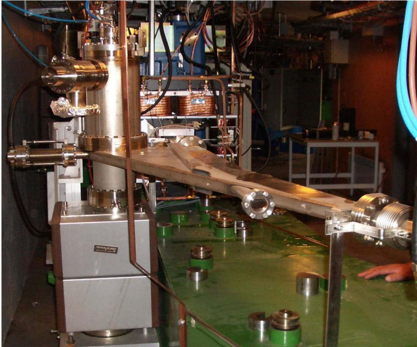
NEG coated dipole chamber of Cu to be tested in MAX II.
