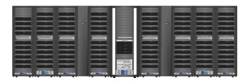
Kalkyl, Intel Xeon E5520, 2784 cores, IB,20 Tflops
