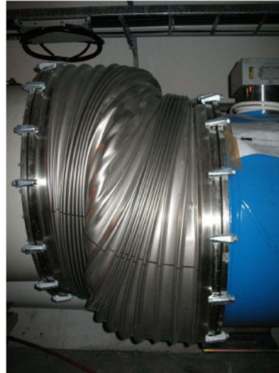
Collateral damage: magnet displacements
