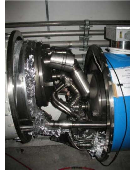
Collateral damage: magnet displacements
