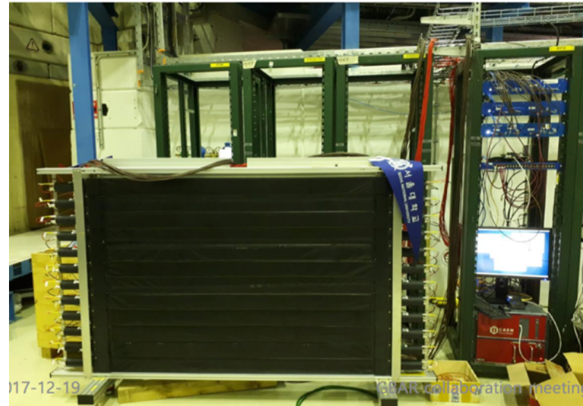
a plane of TOF bars from SNU
