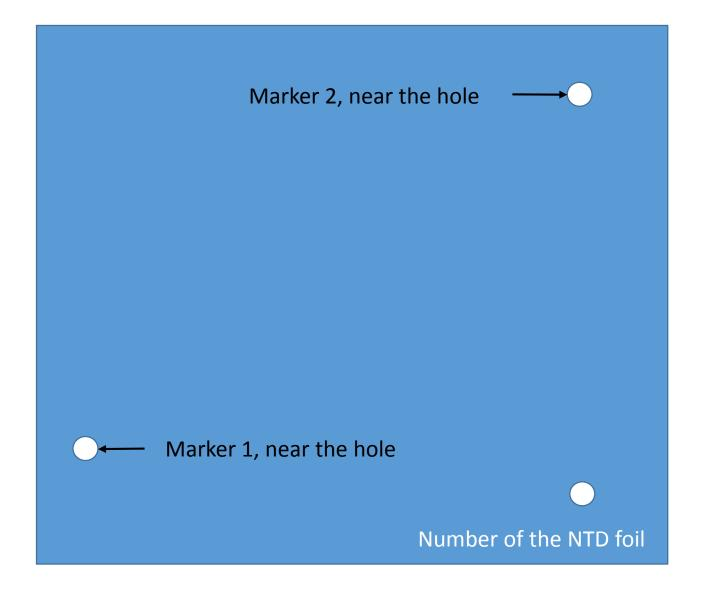
Sketch of a single NTD foil with drilled holes + markers' positions
