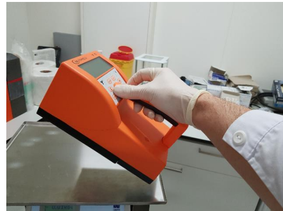
At the end we verify the contamination of surface with an activimeter
