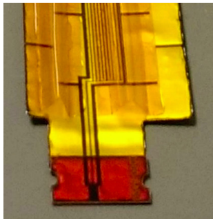
Mock-up ladders made of tape heaters
