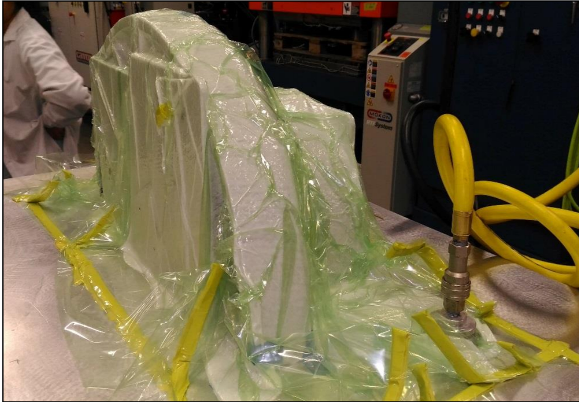
Layup bagged for the oven
