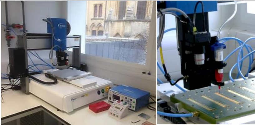
Nordson EFD Pro4 vision guided liquid dispensing robot and Ultimus V controller Cost £30K (ex. VAT)
