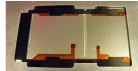
Figure 19: Broken wirebonds between sensors following module transport.
