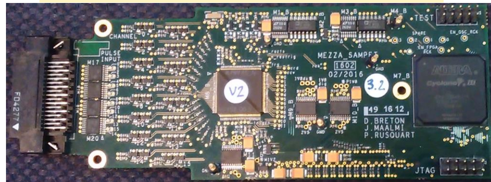
Mezzanine with flat cable differential digital input
