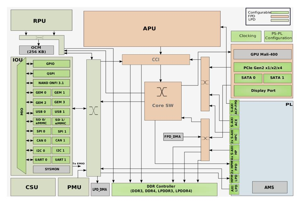
Independent power domains where each sub-system can be powered up, powered down, restarted or suspended without affecting the other sub-systems
