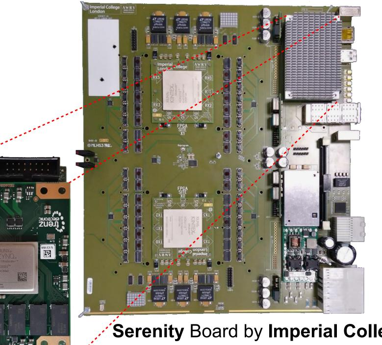
► FPGA logic and high-speed transceivers tightly coupled to processing system
