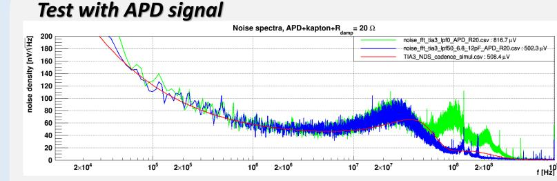
Noise density spectra of CATIA connected to APDs as in ECAL. In green, without bandwidth limitations, in blue with a low pass filter at 50 MHz and in red the simulation results
