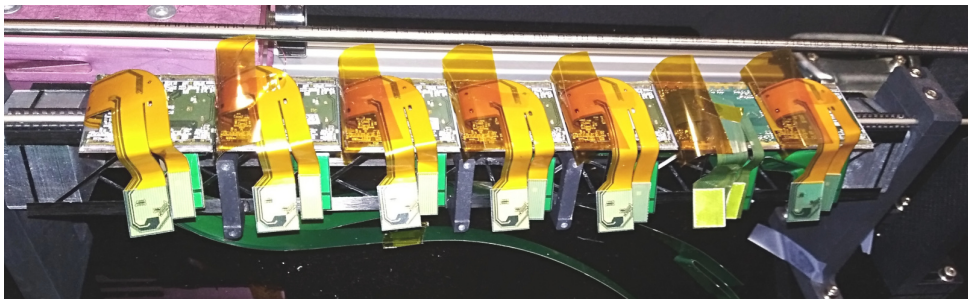
Figure 3: Short electrical prototype with 7 quad modules.
