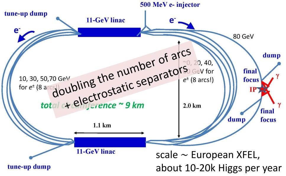
SAPPHiRE: Small Accelerator for Photon-Photon Higgs production using Recirculating Electrons
