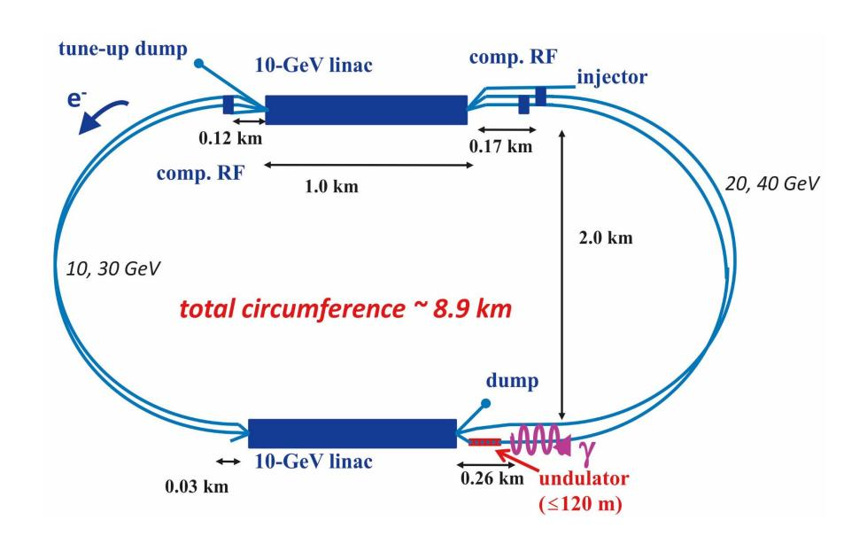
The main LHeC-ERL electron beam parameters.
