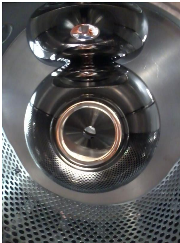
GTS 350 kV In operation since Nov. 2016 with CsK 2 Sb photocathode: 500 uA magnetized beam 4.5 mA non-magnetized
