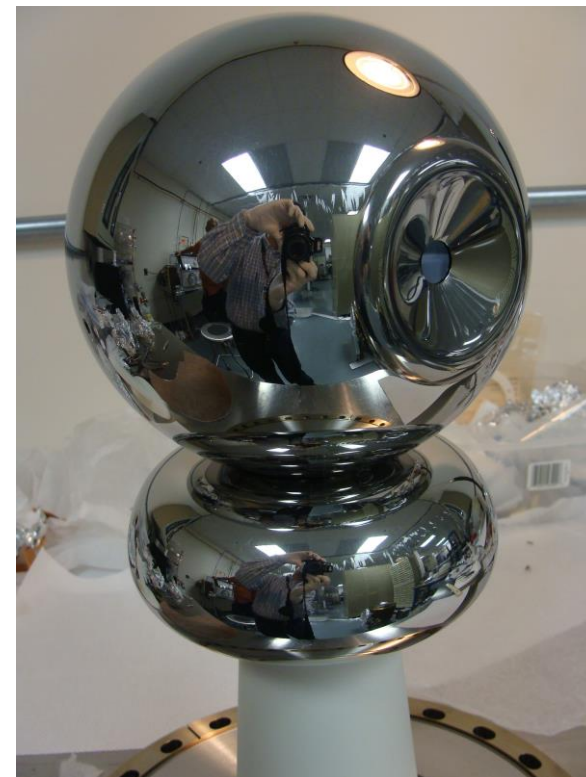
UITF 350 kV Polarized Gun Under assembly
