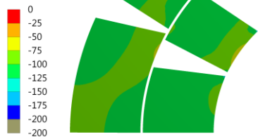
C: DS11T-1in1-non-linear Hoop - conductor Type: Normal Stress(Y Axis) Unit: MPa Cylindrical system Time: 2 Max: -64.988 Min: -148.49
