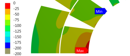
E: DS11T-1in1-2 con collar displaced Hoop - conductor Type: Normal Stress(Y Axis) Unit: MPa Cylindrical system Time: 2 Max: -14.573 Min: -138.91
