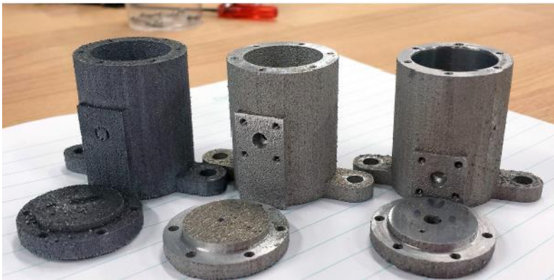
A 3D Printed Superconducting Aluminium Microwave Cavity
