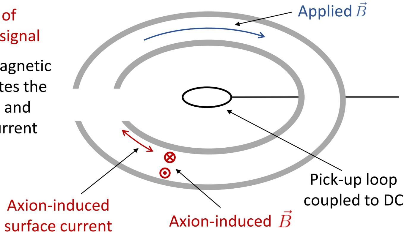
For large  $\omega$ , the current does not propagate to the outside, and the axion-induced signal is screened.
