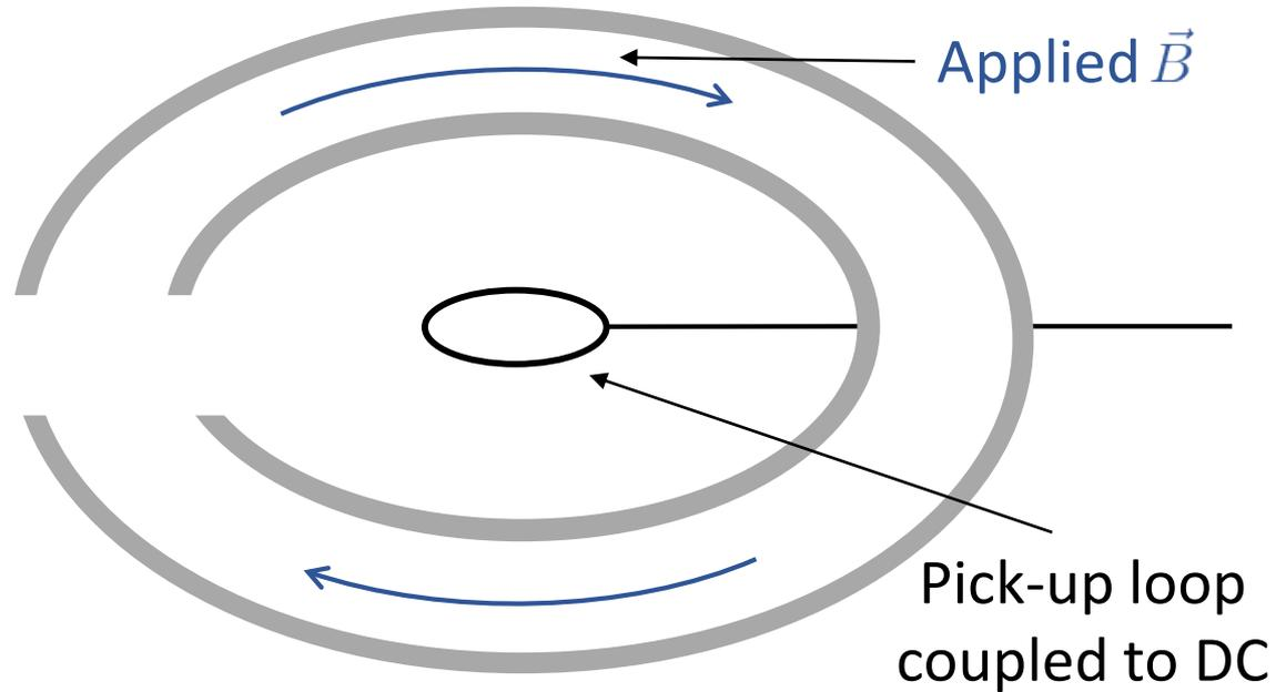
This can be achieved with a “gapped torus”, i.e. a finite open cylinder bent into a torus-like shape without connecting the ends.
