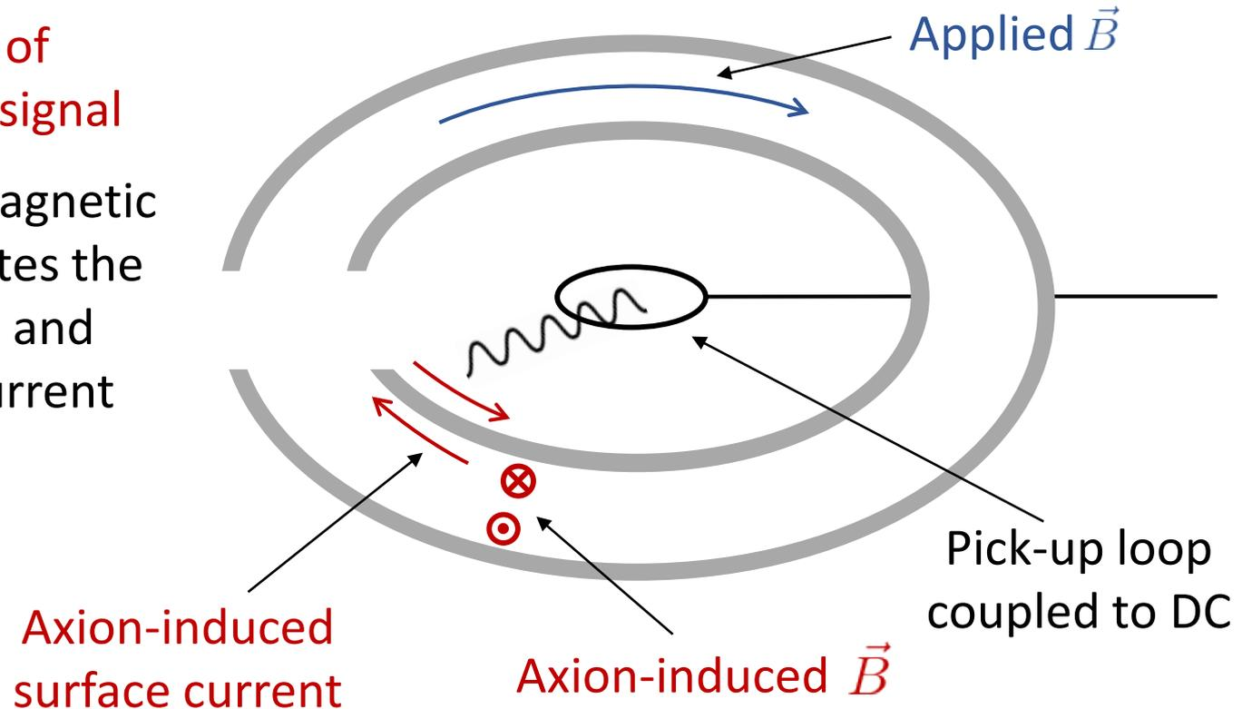
For sufficiently small  $\omega$ , the current continues to the outside of the torus and sources a magnetic field in the central pick-up loop.
