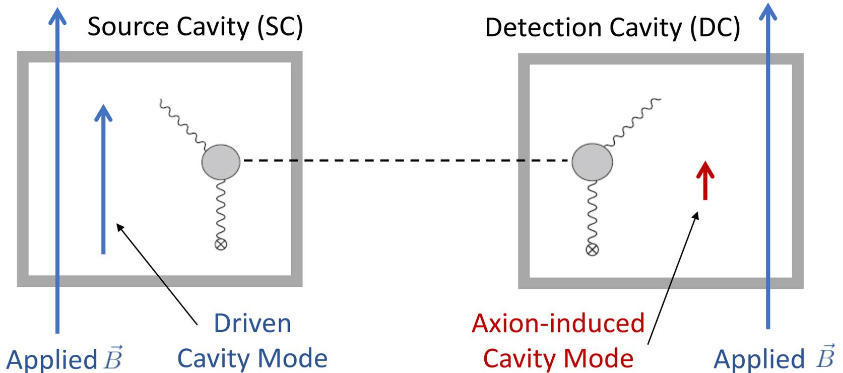
$$P_{\text{signal}} = P_{\text{input}} \cdot \left( \frac{gB}{\omega} \right)^4 Q_{\text{SC}} Q_{\text{DC}} |G|^2$$
