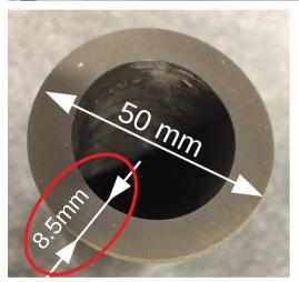
Produced by the Reactive Liquid Magnesium Infiltration (RLI) process
