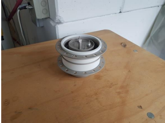
Pseudospark Switch TD11-200K/25 max. 200 kA and 25 kV
