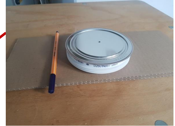
ABB D2601N Diode max. surge current 52 kA, max. 9kV
