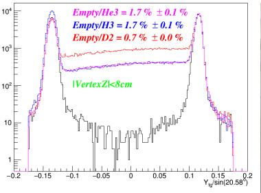
CENTER Image: Shown are the tritium, He, D target data as compared to running on an empty cell (black). The tritium and other gas targets are clearly visible between the aluminum entrance and exit windows of the target cell.
