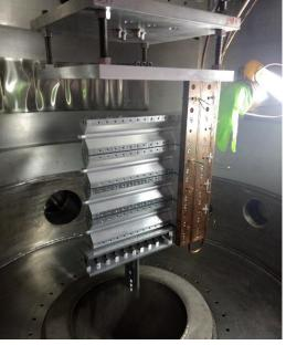
RIGHT Image: The target cell stack during installation in the Hall A scattering chamber.
