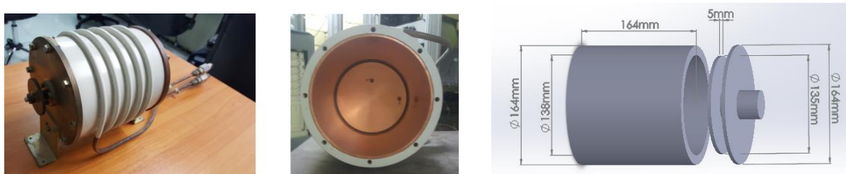
Figure 1. Pictures and drawing of the resonant cavity at the PBP-CMU Electron Linac Laboratory.
