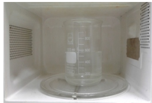
Figure 2. 500 ml of Water in beaker (Pyrex Glass) in Microwave oven in microwave power measurement
