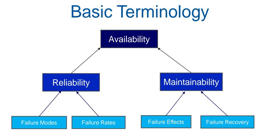
Failure behaviour and recoveries are described by stochastic processes (probability density functions)
