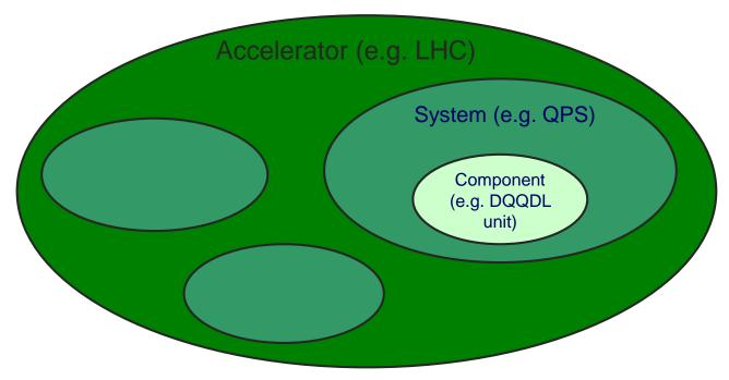
Availability models typically start from accelerator and system levels (repairable systems) and can go down to component level
