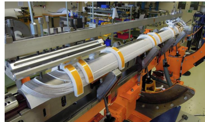
11 T coils during production
