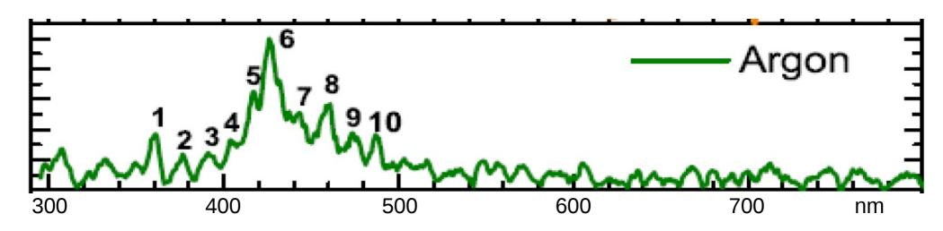
Spectrum obtained at GSI with 4.757 MeV protons
